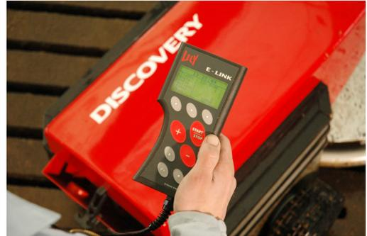
Figure 4 2 E-link manual controller
