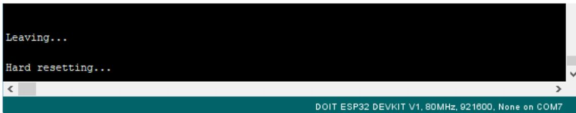
The SPIFFS image has been uploaded to the ESP32 board
