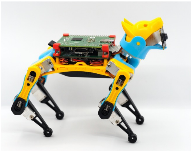
The red Pi standoff can be 3D printed.
