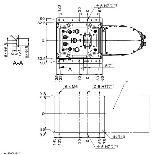
\* Maintenance window: Opening to access inner arm's cover is recommended.
