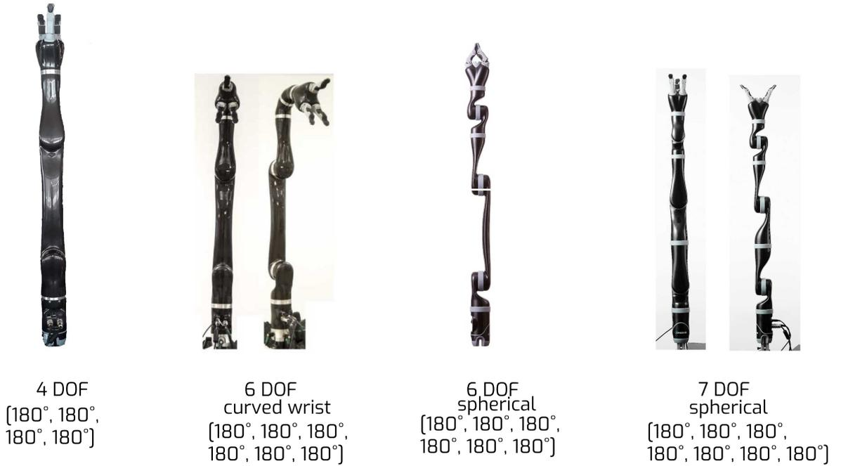
**Figure 2: Set zero positions joint angles**
