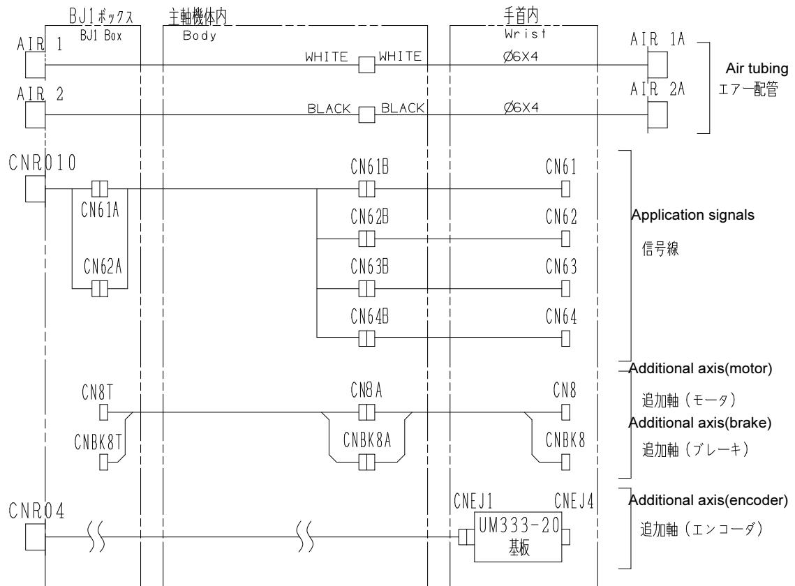
For additional axis encoder, it is necessary to use a bus-connection type encoder that is designated by NACHI. For more details, please contact our technical department.
