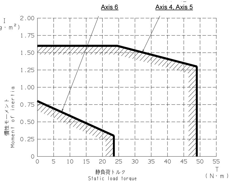
■ How to calculate inertia moment of wrist axes
