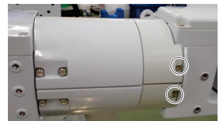
Cross recessed binding head machine screw: 2-M3×6 (×2)
