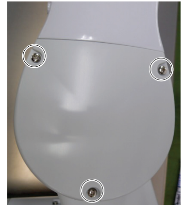
Cross recessed binding head machine screw: 3-M3×6
