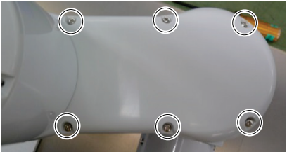
Cross recessed binding head machine screw: 6-M3×6
