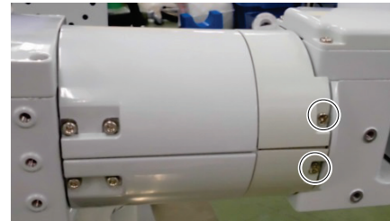
Cross recessed binding head machine screw: 2-M3×6 (×2)
