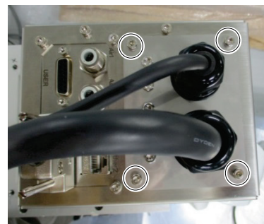
Hexagon socket head cap bolts: 4-M4×8
