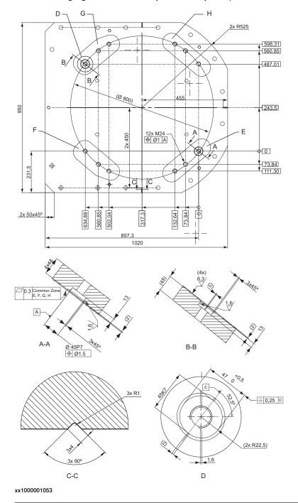
E, F, G, H Common tolerance zone (accuracy all over the base plate from one contact surface to the other)
