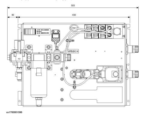
The standard water and air unit consists of four main assemblies.
