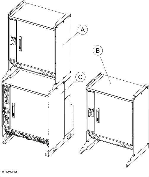
Spot welding cabinet, mounted on IRC5 controller
