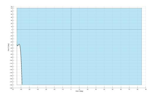
Working range axis 2 and axis 3 for IRB 6700-300/2.70 and -245/3.00 Limited in some areas to avoid collision with balancing.
