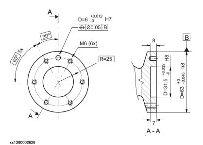
For fastening of gripper tool flange to Robot tool flange every one of the screw holes for 6 screws, quality class 12.9 shall be used. Min. 10 mm used thread length.
