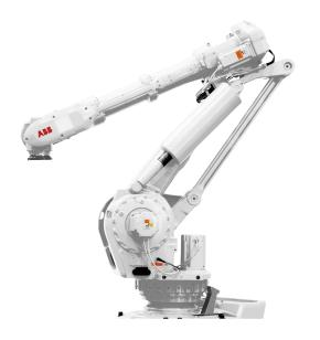
The IRB 6660 is an extremely reliable robot designed for high performance applications. The stiff design supports accuracy and short cycle times, which in the end increases productivity. It comes in three versions, two with long reach aimed at high-performance press tending operations and the third designed for challenging applications like machining of castings.
